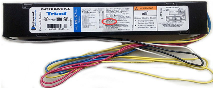
A typical Non-PCB containing fluorescent light ballast. The ballast has a "No PCBs" marking on the top of the ballast and the text "electronic ballast". Only magnetic fluorescent light ballasts contained PCBs.
